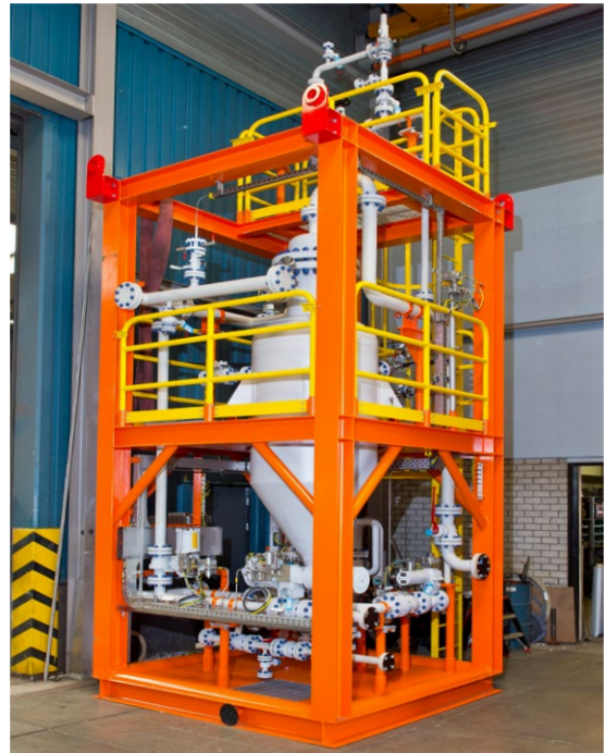
Sand Cleaning Skid
