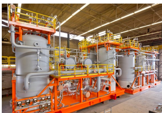
Produced Water Treatment Skid
