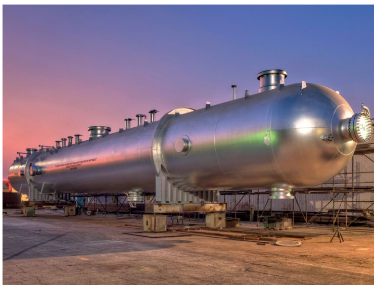
Gas Liquid Separator
