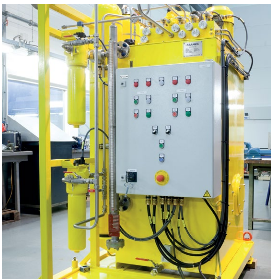
Hydraulic Power Unit
