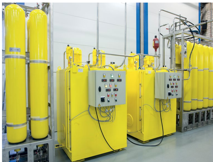
Hydraulic Power Unit
